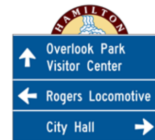
Community Wayfinding Guide Sign with Enhancement Marker
