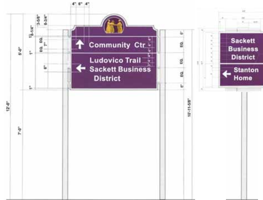
Vehicular Directional Signs - double post mounted on left and single pole mounted on right
