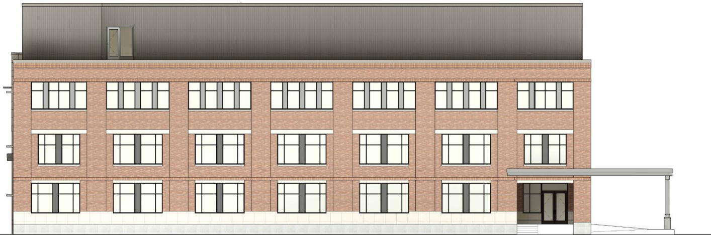
3 EXTERIOR ELEVATION - NORTH 1" = 10'-0"
