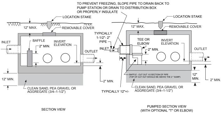
NOTE: BAFFLE MAY BE REPLACED BY A PVC TEE ("T") OR ELBOW
