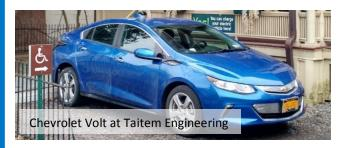
**Plug-in Hybrid Electric Vehicles (PHEV)** have a battery-powered electric motor to drive 15-80 miles then use an internal combustion engine powered by another fuel such as gas or diesel.
