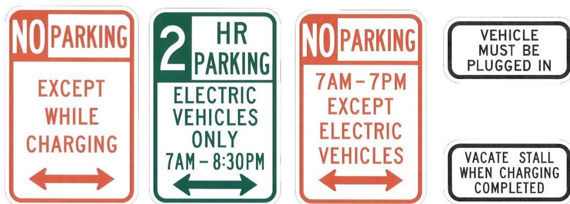
Figure 10: MUTCD recommended regulatory signage
