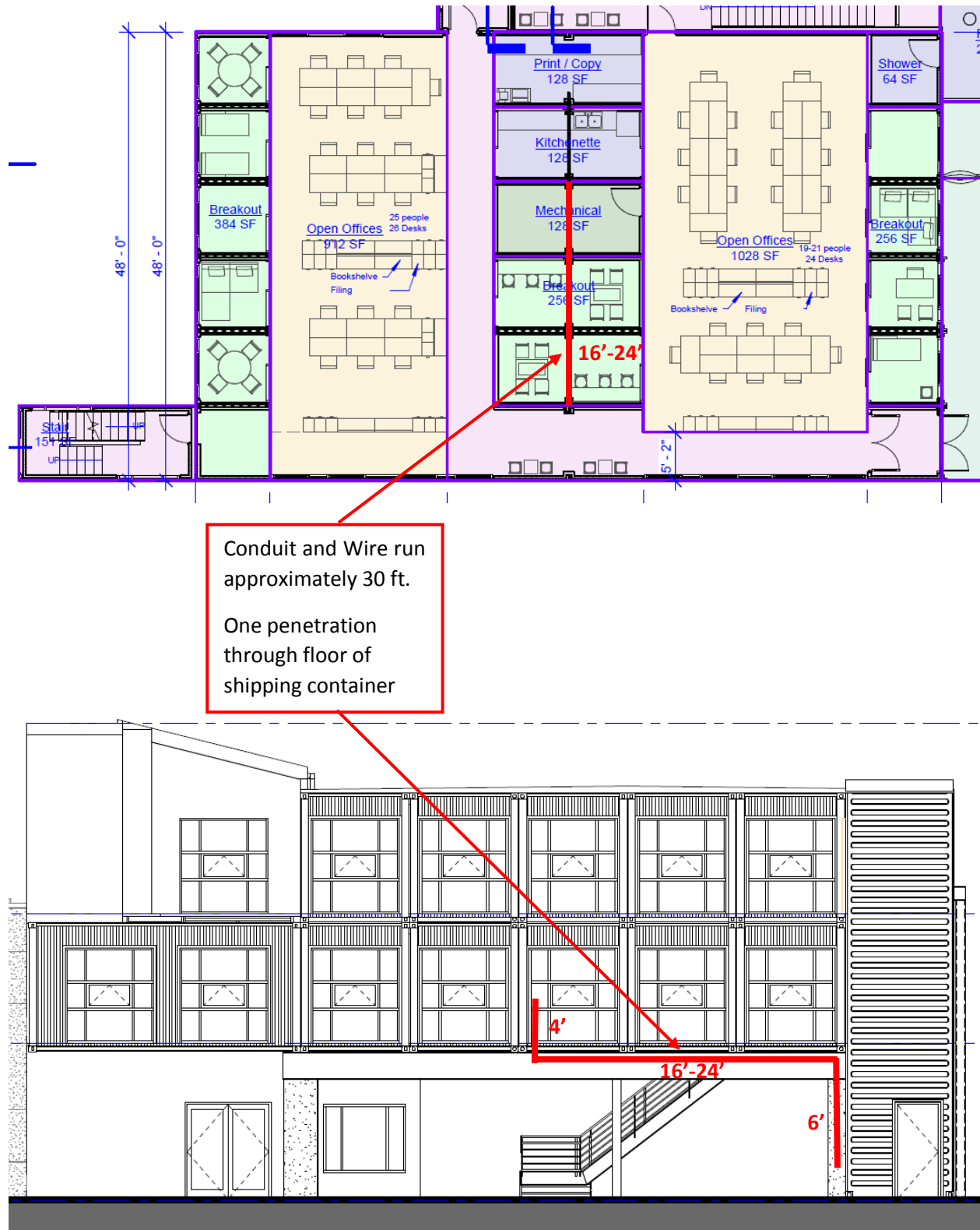
Figure 27. Electrical wiring run for the proposed location for a new charging station at Cornell Cooperative Extension's planned expansion
