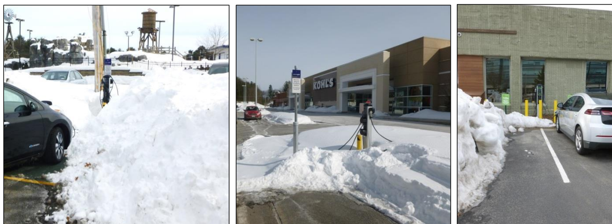
Figure 22: Snow management practices may impede EV charging
